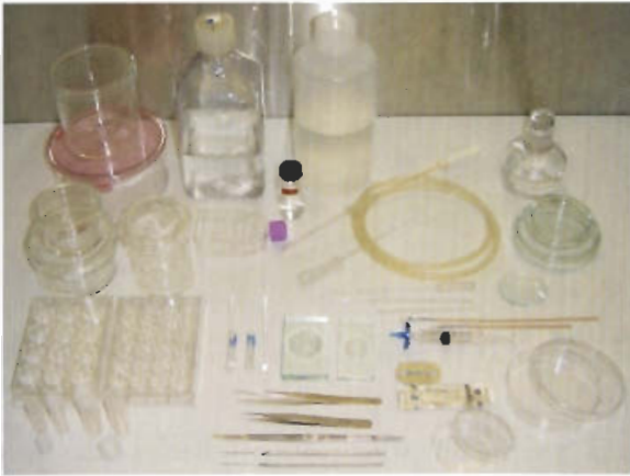
FIGURE 9.1. Tools used for macroalgal cultures (glassware, multiwell dishes, small vials for stocks, plastic containers for medium, Pasteur pipettes with silicone bulbs and tubing, polystyrene transfer pipettes, depression slides, glass homogenizer, forceps, scalpel, needles, paint brushes, syringe with membrane filter cartridge, razor, alcohol lamp, watch glass, and glass and plastic petri dishes).
