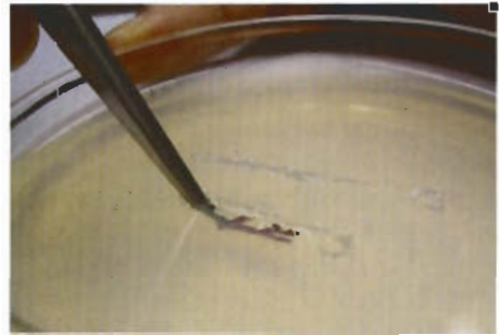
FIGURE 9.7. Cleaning of algal tissue by dragging the fragment through an agar plate.
