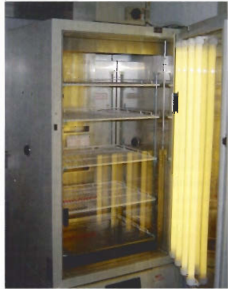
FIGURE 9.2. Incubators converted from cooling incubators by adding lighting units (fluorescent tubes and a timer controlling the lighting; the ballasts should be mounted outside the chamber).
